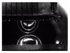
These observations were also combined with observations of two parallel modified glass surfaces with varying distance between them (fig.7). In this case studies of water drops coalescence events can be combined with influence of varying distance between walls.
